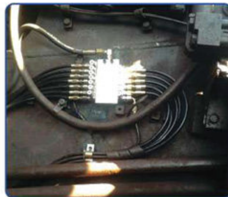
Mono Block Progressive Distributor Performance indicator Type fitted at the bottom of the Dumper to find the exact bearing blockage if any
