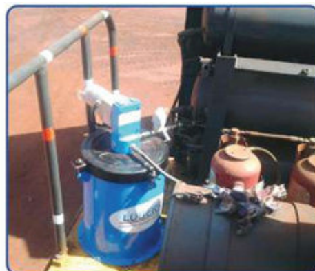
MOTOLUBERR DC operated pump mounted on Top of the Dumper
