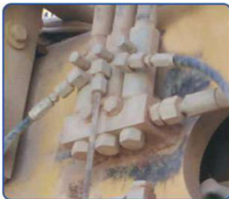
Grease Injector SVM 01 fitted on the Dumper
